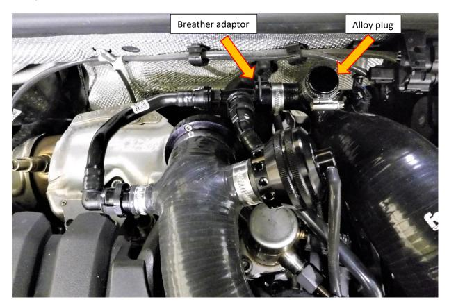
If your vehicle is not equipped with the extra breather hose, use the remaining alloy blanking plug to block off the spout and secure with the 16-27 hose clamp.
