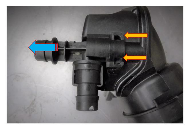
6. With the breather adaptor now removed, take the Forge Motorsport billet breather adaptor, and push it onto the end of breather adaptor with the green O ring. There is location marker on the billet adaptor which must be lined up with the plastic moulded line as shown in the picture below. Use the U clip supplied to secure the billet adaptor in place.
