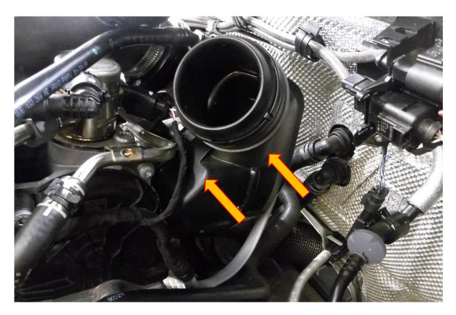
5. With the use of long nose plyers push in the two tabs while pulling the adaptor to free it. Remove the breather hose adaptor from the OE turbo elbow.
