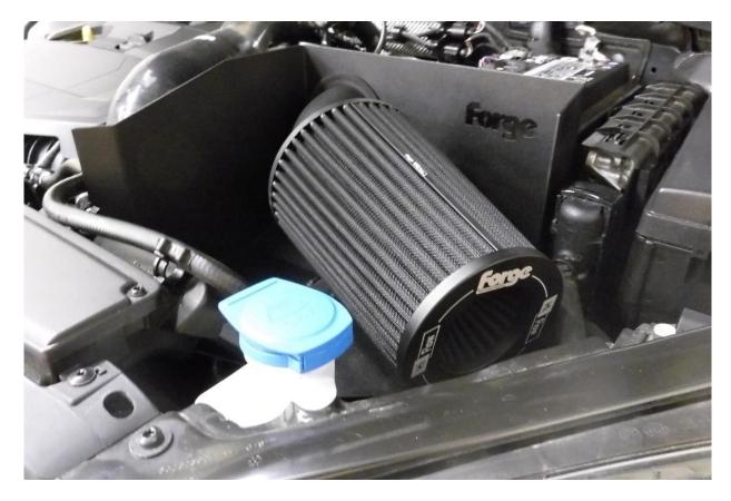
On certain vehicles with the washer spout is in the location below, you may have to position the air filter further down the alloy intake pipe.
