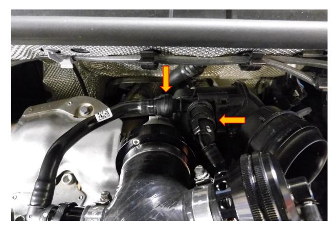
4. Using a T30 rachet and suitable extension remove the two T30 fasteners attaching the OE turbo elbow to the turbo charger.
